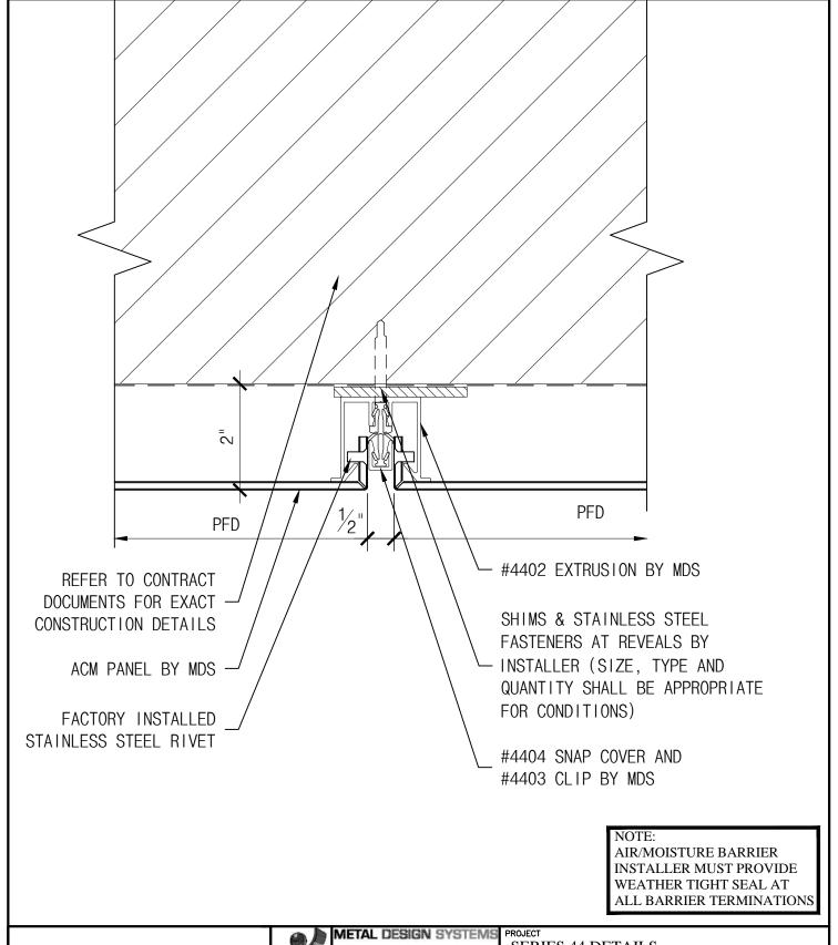
THE INFORMATION CONTAINED IN THIS DRAWING IS THE SOLE PROPERTY OF METAL DESIGN SYSTEMS. ANY REPRODUCTION, IN PART OR WHOLE, WITHOUT THE WRITTEN PERMISSION OF METAL DESIGN SYSTEMS IS PROHIBITED. DESIGN SYSTEMS
