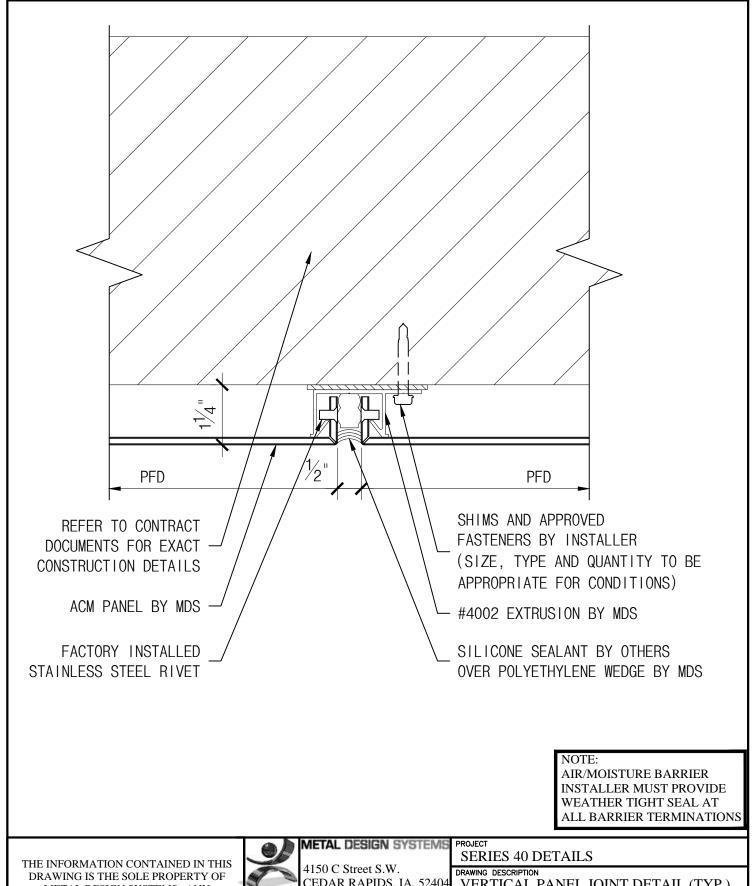
CEDAR RAPIDS, IA. 52404 VERTICAL PANEL JOINT DETAIL (TYP.) METAL DESIGN SYSTEMS. ANY Ph. (319) 362-7454 DRAWING NUMBER S40-ACM-04 REPRODUCTION. IN PART OR WHOLE. PROJECT NUMBER WITHOUT THE WRITTEN PERMISSION OF DESIGN SYSTEMS METAL DESIGN SYSTEMS IS PROHIBITED. MATERIAL SCALE DRAWN BY 6" = 1'-0"
